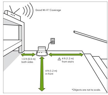
**MARNING:** To prevent the risk of your robot falling downstairs, ensure that the dirt disposal is placed at least 4 feet (1.2 meters) away from stairs.
