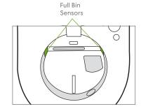
Remove the filter and wash the bin, or gently clean the bin to ensure the sensor ports are clean.
