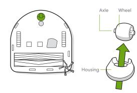
\* Important: A rear wheel clogged with hair and debris could result in damage to your floor. If the wheel is not could result in damage to your floor. If the wheel is not spinning freely after you have cleaned it, please contact Customer Care.
