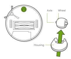
Important: A front wheel clogged with hair and debris could result in damage to your floor. If the wheel is not spinning freely after you have cleaned it, please contact Customer Care.
