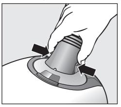
Press the release buttons at the side of the hose connector, and lift the hose from the socket.
