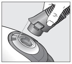
Insert the hose connector into the suction socket on the vacuum cleaner until it clicks into position. To do this, line up the guides on the two pieces.
