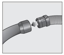
■ Fit the connector at the other end of the suction hose into the handle until it clicks into position.
