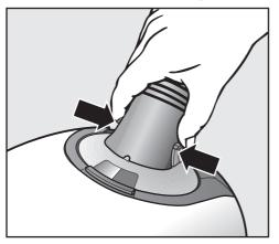
Press the release catches at the side of the hose connector, and remove the hose from the socket.
