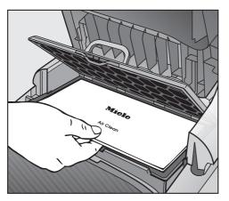
Replace it with a new AirClean exhaust filter.
