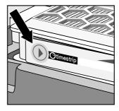
Press the TimeStrip® exhaust filter change indicator.
