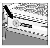
■ If you are using exhaust filter **c** or **d**, press the TimeStrip® exhaust filter change indicator.
