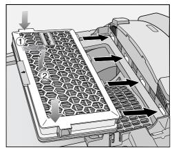
■ Insert a new exhaust filter, making sure it goes in properly, then push it down into position.
