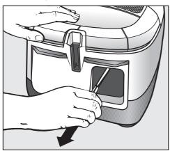
■ Pull the power cord out to the required length (max. cord length approx. 21" (6.5 m).
