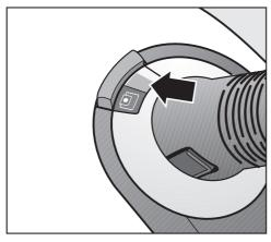
Change the FilterBag when the color marker in the FilterBag change indicator turns red.
