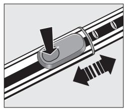
Press the release button and adjust the telescopic suction wand to the required length.
